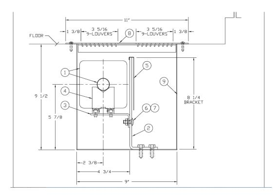
NOTE: The above drawing is for reference only. Each trough installation is based on individual job conditions. Also, make sure that the element is installed on the room side of the trough.
